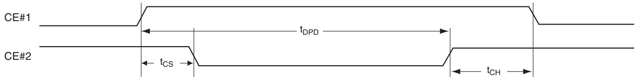
Figure 32. Deep Power-down Timing
